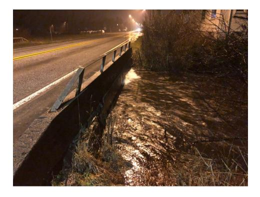
The culvert under the road is full and a further increase in water flow would have catastrophic consequences for more homes. Flood in Øyebekken in Kvinesdal.
