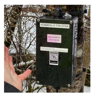
Data from Breibekken is collected in the watertight plastic box, easily mounted, where the battery must be replaced every three weeks.
